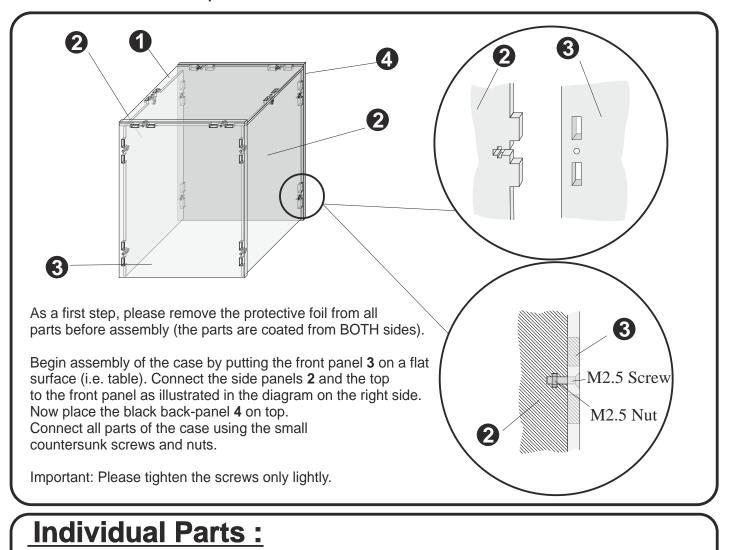
1 x Set of Screws for Case and Ball-Stand (20 x M2.5 Countersunk Screw, 20 x M2.5 Hexagon Nut) 1 x Set of Screws for the Base (2 x Screw M4 x 6mm, 2 x Sleeve Nut M4 x 7mm)
