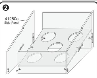
Once the first side-panel is connected with the front-, back-, and golfball-support-panel, take the second side-panel and fix it to the opposite side using the small countersunk-screws and nuts.
