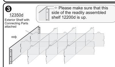
Connect the two readily assembled shelves 12350d, to the side panels 12350b using the small M3 screws and nuts.
