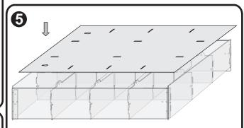
Finally connect the back panel to the sides and shelves. Clamp it firmly with the acrylic wedges. To interconnect several BD Racks or BD, CD and DVD racks sideways please use the longer M3 screws and nuts.
