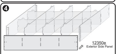
Now connect the two exterior side panels 12350e to the shelves and also to the connecting parts.
