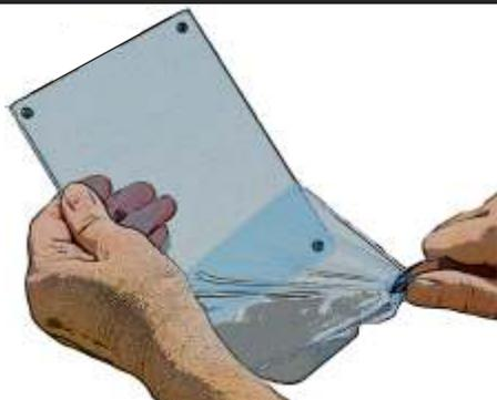
All acrylic parts are coated with a protective foil on BOTH sides. This foil has to be removed before the assembly. We suggest to have a microfiber cloth ready to clean the surface, if necessary.
