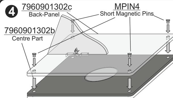
Place the back-panel with the attached frame-stand on top of the front-panel and centre part.
