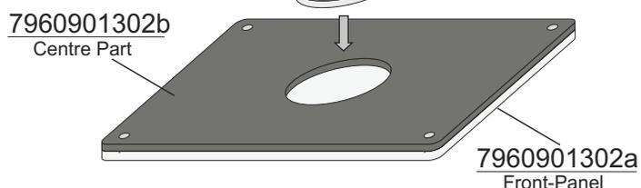
Now place the black centre part with the cut-outs on top of your transparent front-panel and centre panel. Place your coin inside the cut-out in the black centre part.
