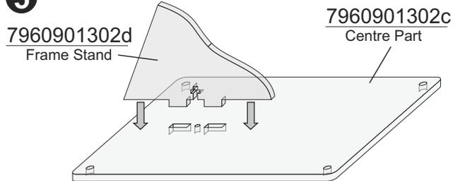
Slot the frame-stand into the back-panel of the frame, as indicated. Make sure that countersunk side of the back-panel is opposite to the frame-stand.
