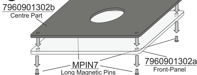
Place the long magnetic pins on a flat surface with their shafts pointing up. Align them like the holes in the transparent front-/back panel. Now put the front-panel on the magnetic pins. Place the centre part on top as indicated.
