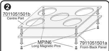
Place the long magnetic pins on a flat surface with their shafts pointing up. Align them like the holes in the transparent front-/back panel.
