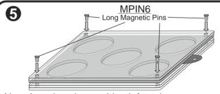
Now there is only one thing left to do: Slot the 4 long magnetic pins through the holes In the front- and center panel. They will instantly snap to their magnetic counterparts.
