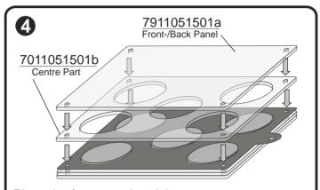
Place the front panel and the transparent centre of the assemble lower part of the case as indicated.
