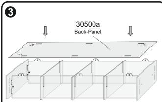
Finally connect the back panel to the sides and shelves. Clamp it firmly with the acrylic pegs.
