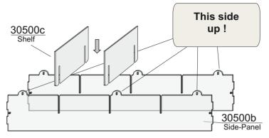
Slot the shelves 30500c (two pieces) into the side panels 30500b. Make sure that the round overlaps with the openings are up.
