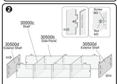
Connect the two Exterior Shelves 30500d, to the side panels 30500b using the small M3 screws and nuts. Please fasten the screws only lightly.
