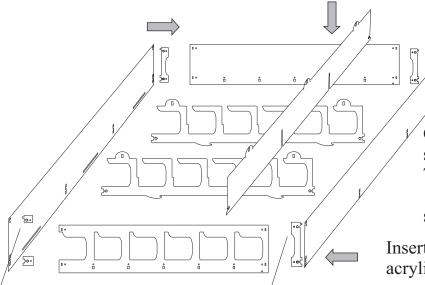
Please remove the protection film from the acrylic sheets before assembling. At first, please connect the five interior shelves to the side panels.
