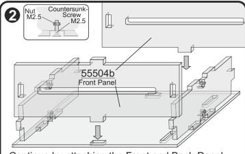
Continue by attaching the Front and Back-Panel 55504b and connecting the Side-Panels to to the Bottom-Panel using the small countersunk M2.5 screws and nuts. Do not overtighten the screws.
