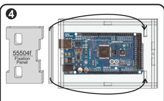
As a final step, take the Fixation-Panel with the holes pointung to the top and slot it into the small holes inside the bottom panel. This will hold the Support Panel in place and clamp your Arduino board to the case.
