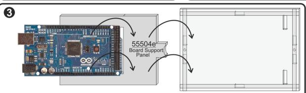
Now put the Board-Support Panel inside the MEGA case as illustrated. Place your Arduino on top of the support panel and guide it carefully through the cut-outs in the Side-Panel
