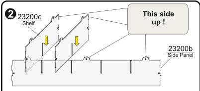
Slot the shelfs 23200c on the side panel 23200b. Make sure that the round overlaps with the openings are up.
