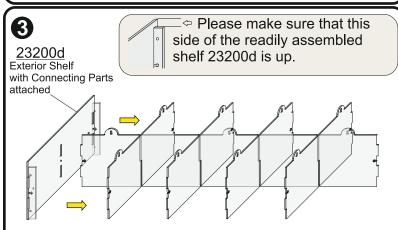
Connect the two readily assembled shelves 23200d, to the side panel 23200b using the small M3 screws and nuts.
