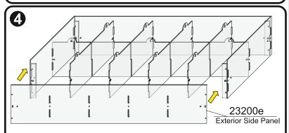
Now connect the two exterior side panels 23200e to the shelves and also to the connecting parts.
