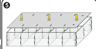
Finally connect the back panel to the sides and shelves. Clamp it firmly with the acrylic pegs. To interconnect several CD Racks or CD and DVD racks sideways please use the longer M3 screws and nuts.
